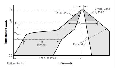
Note: All temperatures refer to topside of the package, measured on the package body surface.
