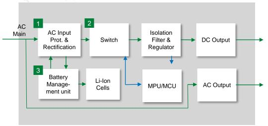
Legend: → Power Line Signal Line USB outlet operates as a switch mode power supply
